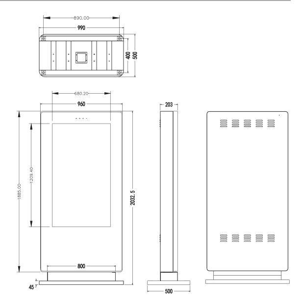
Note: The Ø30 holes are for access, we recommend using M10 anchor bolts that will fit into the Ø16 holes.
