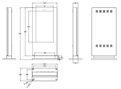
Note: The  $\emptyset$ 30 holes are for access, we recommend using M10 anchor bolts that will fit into the  $\emptyset$ 16 holes.
